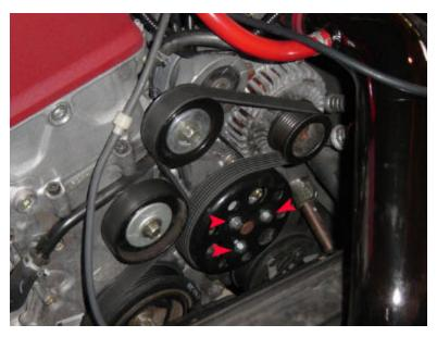
**Figure 1 Water Pump Pulley Bolts**
