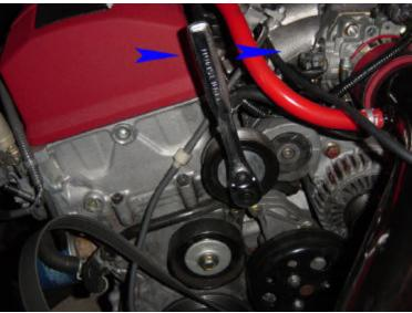
**Figure 3 Auto-Tension Pulley Removal**
