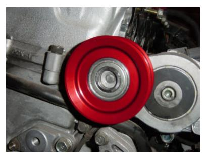
Figure 4 Auto-Tension Pulley Replaced
